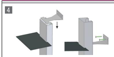
insert wall bracket at top of stem. with stak in final position, fasten the bracket to the wall. this ensures stability.
